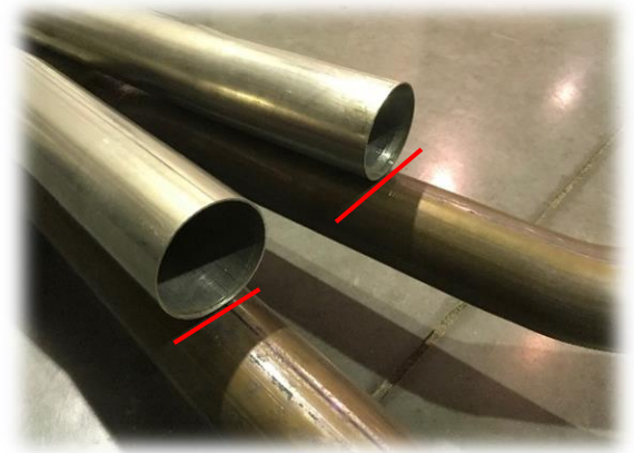
Figure 2 Markings for cutting on factory exhaust
